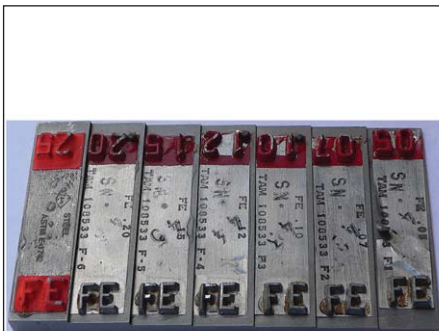
Fig. 4a: Step wedge of steel with ASTM E 1025 IQIs for determination of image quality.
