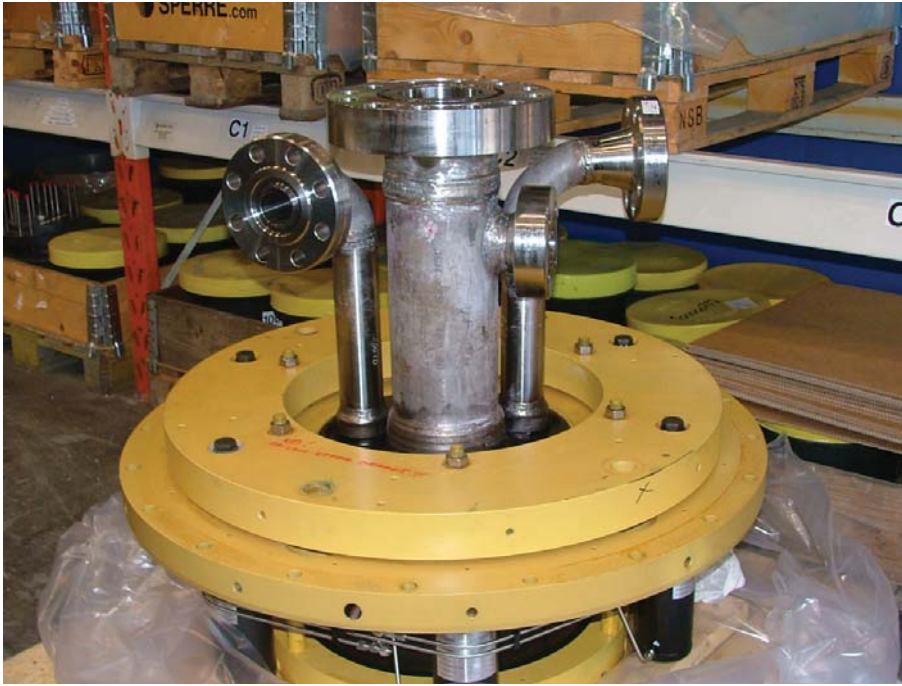
NDT utfordringer, x-mas tree connector
