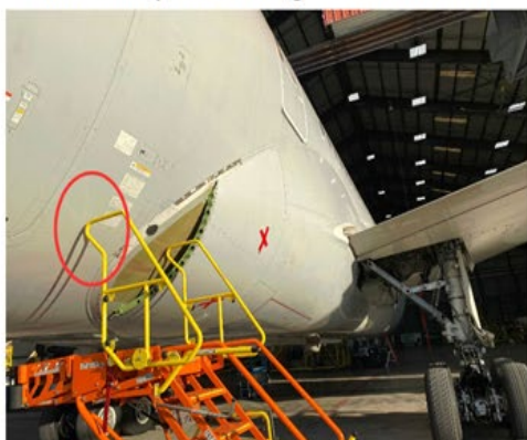
Aircraft Impact Damage - Delamination
